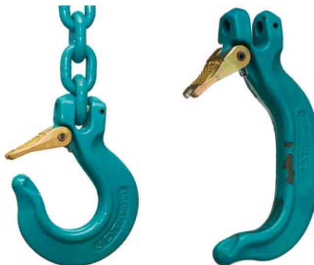
JDT clevis sling hooks are designed in such a way that in the case of overload they NOT break brittle, but hook aperture visually opens and lets the load slowly slide down.
